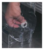
1. Replace the auger nose bushing inside the front of the hopper.
