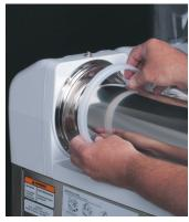
5. Remove the hopper seal from the flange on the cooling drum.
