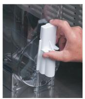
7. Carefully slide valve up to remove spring and faucet seal. Extra care should be taken when handling the seal to prevent damage.
