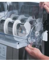
4. Install the hopper over the auger and cooling drum and slide it into place. Push down until the hopper lock plunger snaps into place.
