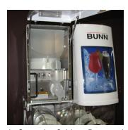
1. Open the Cabinet Door and allow the support arms to lock in place.
