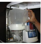
2. Slide the gate shut on the powder hopper and remove the hopper. Remove the Cover and empty the contents.
