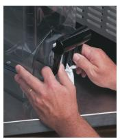
6. **CAUTION:** Faucet valve is under spring tension. Spread one side of the handle first, then the other and disconnect from hopper.
