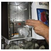
3. Pull the Mixing Chamber out of the Whipper Chamber.
