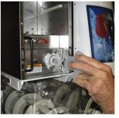
4. Twist the Whipper Chamber clockwise and pull it off the Whipper Chamber Receptacle.
