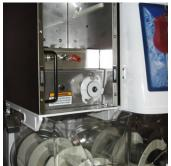
6. Twist Whipper Chamber Receptacle clockwise and pull it off the Motor Shaft. Wipe down all inside surfaces.
