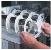
4.Pull the auger from the cooling drum.
