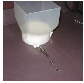
5. Remove the Auger Drive Shaft by turning the screw of the Auger Drive Bracket in a **clockwise** direction.
