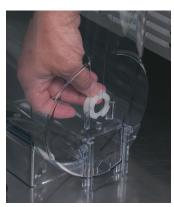
8. Remove the auger nose bushing from inside the front of the hopper. **NOTE:** Do not scratch this surface when cleaning. Deep scratches could cause leakage around the seal.
