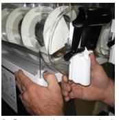
2. Depress the hopper lock plunger, lift slightly.
