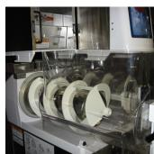
3. Pull the hopper assembly forward and remove.
