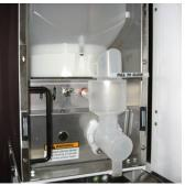
2. Place the power switch in the OFF position. Slide the gate shut on the powder hopper and remove the hopper. Wipe the hopper tray clean of powder residue.
