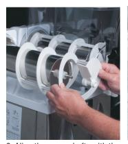
3. Align the auger shafts with the augers. Push the augers as far as they will go and rotate them so the flat face of the auger shaft is aligned with the flat face of the auger nose.
