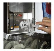
5. Pull the Frother off the Motor Shaft. Notice the flat keyway on the shaft and the matching keyway inside the Frother. It is important that these two keyways are lined up when reassembling.
