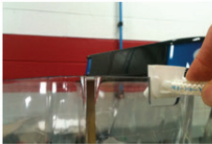
27. Slide hopper fitting into place in the slot on the hopper.
