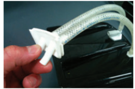
26. Route the tubes from the motor cover together and connect to hopper fitting.
