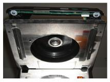
**Step 6**: After the board is reinstalled run a bead of silicon caulk along the front edge near the circuit board.
