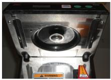
**Step 5**: The black plastic housing can now be lifted up enough on the front to access the two mounting screws for the control board.
