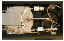
Step 3: Remove two nuts on the inside near the display board.
