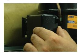
Step 4: Release the harness restraint by removing the screw and pulling the restraint outward and out of the way.
