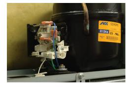
**Step 5**: Locate blue/black wire and install amp clamp around wire. Reconnect power and wait for 6 minute time delay before compressor is activated. Monitor the run load amperage. The run load amp range can be 2.3 to 3.0 amps.
