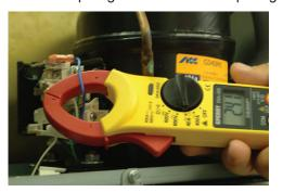
Step 6: If no amperage is present, check for 120VAC across blue/black (hot) wire and white (neutral) on the ptc relay.
