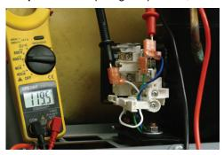
If 120VAC is present then check compressor overload. Unplug machine and check overload for continuity. For instructions on removing or testing the overload and ptc relay review the JDF-S Testing Compressor Overload and PTC Relay instruction sheet.
