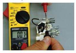
If 120VAC is not present then go back to the compressor relay and check for activation of the relay after 6 minute delay from initial power up.
