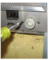
**Step 11**: Place cabinet back onto frame and attach all screws. Screw the top of the board housing onto the cabinet bracket. Reconnect the door harness to its original locations.
