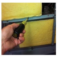
• Remove screws (4) that hold the stainless door wrap to the left and right front frame.
