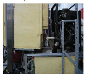
**Step 5:** Separate the water tank lid from the foamed bath.
