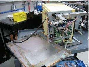
Step 8: Pull the old water tank out from the bottom of the unit. Replace water bath with a new one.
