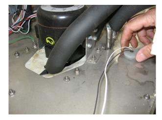
**Step 10**: Replace the rivets with screws and nuts. Re-attach bottom plate to frame with screws. Re-attach circuit board mount to the left side of the base plate. Screw inlet water valve to bracket and re-attach bracket to frame.
