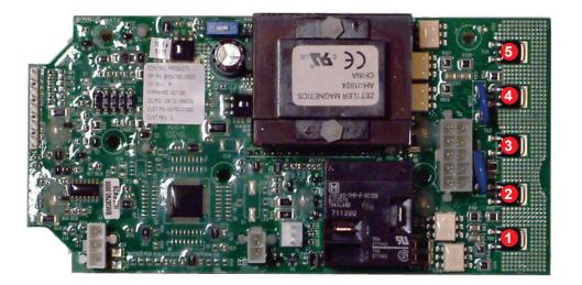
Viewing the Control board as if were installed in the machine on the right vertical edge a series of 5 triacs can be found. They are labeled TH1 to TH5 with TH1 being located at the bottom of the board and TH5 at the top.
