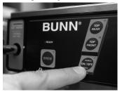
7. Return the brewer to level. Restore power to the brewer. Turn ON the main warmer to allow the tank to refill. Check for leaks around the faucet.
