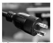
1. Disconnect power from the brewer and allow faucet to cool to touch (could take several hours). NOTE: It is not necessary to disconnect the water source for this procedure.
