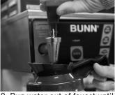
2. Run water out of faucet until flow stops. Elevate the front of the brewer about 1" so water is confined to tank.
