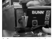
8. Run water through the faucet until no signs of dislodged lime scale are visible.
