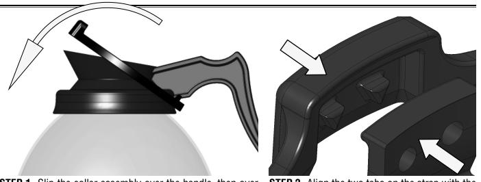
**STEP 1.** Slip the collar assembly over the handle, then over the neck of the decanter.
