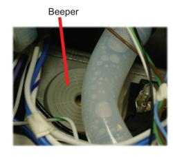
The beeper harness and lock nut can be accessed through the front panel and the beeper is removed from the top or hood assembly.
