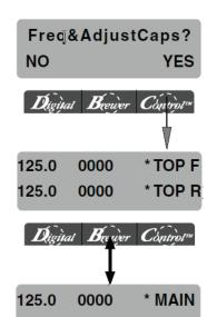
This screen allows the user to monitor the frequency of the RFID coils. It can also be used to monitor the adjustment capacitors, which are used to keep the coil frequency at it's nominal value (125.0 khz).
